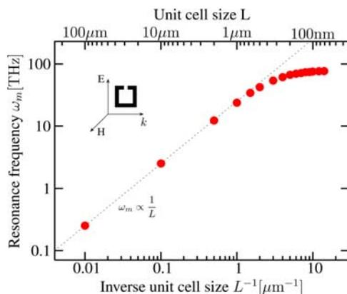
**Fig. 1** (online colour at: [www.pss-b.com](http://www.pss-b.com)) Scaling of the magnetic resonance frequency of the single-cut SRR with the inverse unit size is shown. The parameters of single-cut SRR are given by length  $l = 0.8L$ , width  $w = 0.1L$ , thickness of the metal  $t = 0.05L$  and gap-size  $g = 0.02L$ . The linear scaling  $\omega_m \propto 1/L$  at low frequencies (large unit cells) breaks down at around 100 THz.
