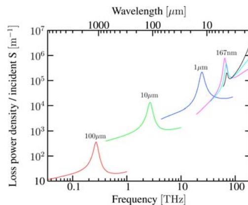
**Fig. 4** (online colour at: [www.pss-b.com](http://www.pss-b.com)) Loss power density per incident power flow density (Poynting vector) is shown across the magnetic resonance for the different single-cut SRR sizes from Fig. 1.
