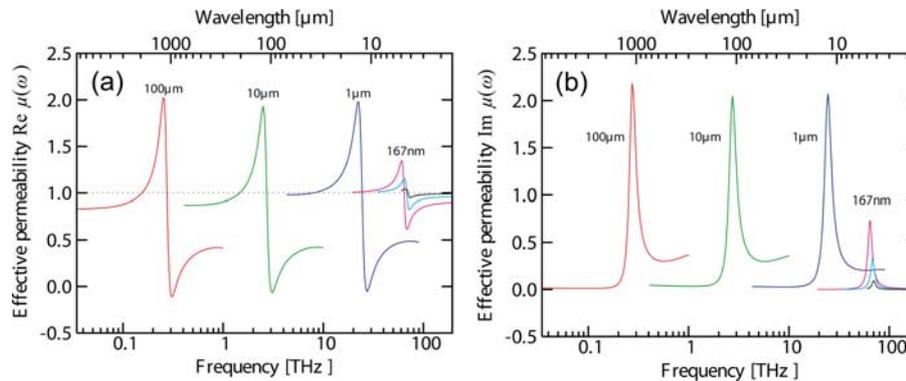
**Fig. 2** (online colour at: [www.pss-b.com](http://www.pss-b.com)) Real part (a) and imaginary part (b) of the resonant effective permeability  $\mu(\omega)$  are shown for a single-gap SRR as function of frequency for different sizes  $L$  of the SRR unit cell:  $L = 100 \mu\text{m}$  (red),  $10 \mu\text{m}$  (green),  $1 \mu\text{m}$  (blue),  $167 \text{ nm}$  (pink),  $100 \text{ nm}$  (turquoise) and  $50 \text{ nm}$  (black).
