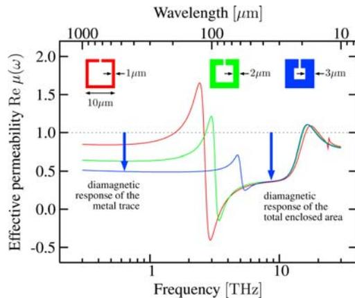
**Fig. 5** (online colour at: [www.pss-b.com](http://www.pss-b.com)) Real part of the effective magnetic permeability  $\text{Re}(\mu(\omega))$  is shown around the magnetic resonance for a fixed SRR size of  $10\ \mu\text{m}$  and different widths of the metallic ring. Note the diamagnetic response of the metal area (left, below resonance) and the total enclosed ring area (right, above resonance).
