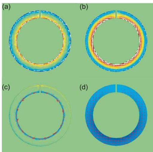
**Fig. 6** (online colour at: [www.pss-b.com](http://www.pss-b.com)) Current distribution inside the SRR is shown for the diamagnetic response below the magnetic response at (a) 300 GHz (SRR size  $L = 10\ \mu\text{m}$ ); and (b) 30 THz (SRR size  $L = 100\ \text{nm}$ ); as well as for the resonant response of (c) 3 THz ( $L = 10\ \mu\text{m}$ ), and (d) 116 THz ( $L = 100\ \text{nm}$ ).
