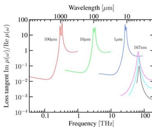
**Fig. 3** (online colour at: [www.pss-b.com](http://www.pss-b.com)) Magnetic loss tangent  $\text{Im } \mu(\omega)/\text{Re } \mu(\omega)$  is shown for a single-gap SRR as a function of frequency for different sizes  $L$  of the SRR unit cell:  $L = 100 \mu\text{m}$  (red),  $10 \mu\text{m}$  (green),  $1 \mu\text{m}$  (blue),  $167 \text{ nm}$  (pink),  $100 \text{ nm}$  (turquoise) and  $50 \text{ nm}$  (black).
