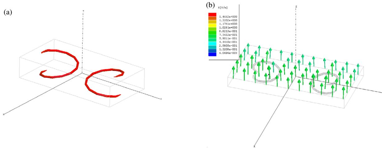
**Figure 7.** Unit cell with a left-handed and a right-handed coil in the  $y$ -direction (a), eliminating the effect of the field rotation (b). The linear polarization of the electric field parallel to the axis of the coils is maintained through the structure. The dispersion relation and plasmon frequency for the principal propagating modes remain essentially unaltered. However, the field eigenmodes are dramatically changed.
