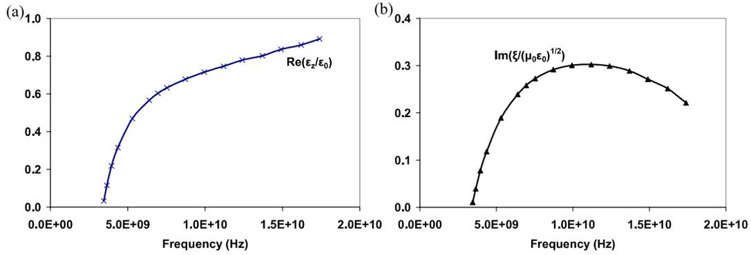
**Figure 5.** The overall material properties of the left-handed coil medium, normalized with respect to the permittivity of free space: the real part of the axial permittivity (a) and the imaginary part of the chirality parameter (b).
