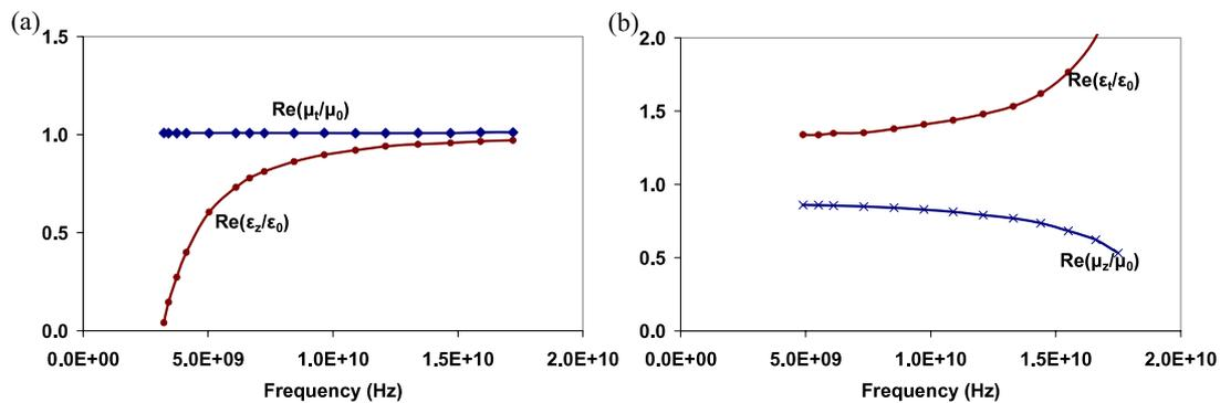
**Figure 8.** The overall material properties of a periodic array of alternating left-handed and right-handed coils. The unit cell and an eigenmode solution for axial polarization are shown in figure 6. (a) The axial permittivity and the transverse permeability related to the axial eigenmode. (b) The transverse permittivity and axial permeability related to the transverse eigenmode
