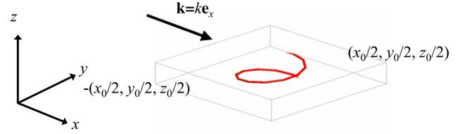
Figure 2. A rectangular cubic unit cell of a uniaxial periodic coil array.
