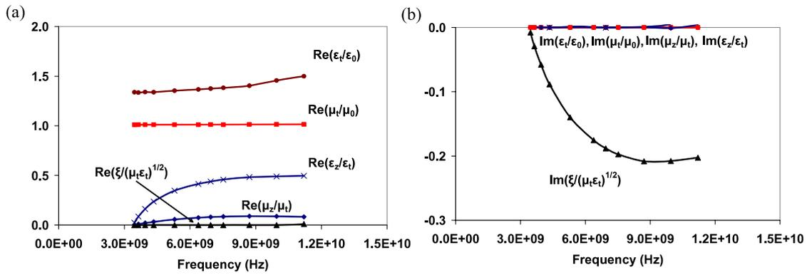
**Figure 6.** The overall material properties of the right-handed coil medium: the real part (a) and the imaginary part (b) of all five parameters. A unit cell consisting of two coils in the  $x$ -direction is used for this calculation. The agreement with the single unit cell (figure 4) is apparent.
