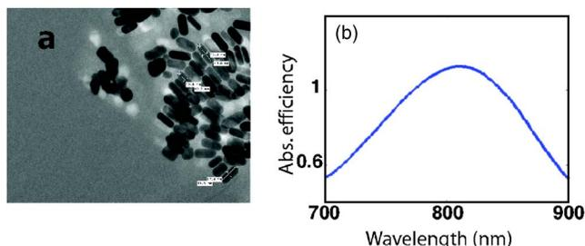
FIG. 1. (Color online) TEM image of a sample of gold nanorods (a) and optical absorption efficiency (single particle absorption cross section normalized by its geometrical cross-sectional area) of the sample (b).
