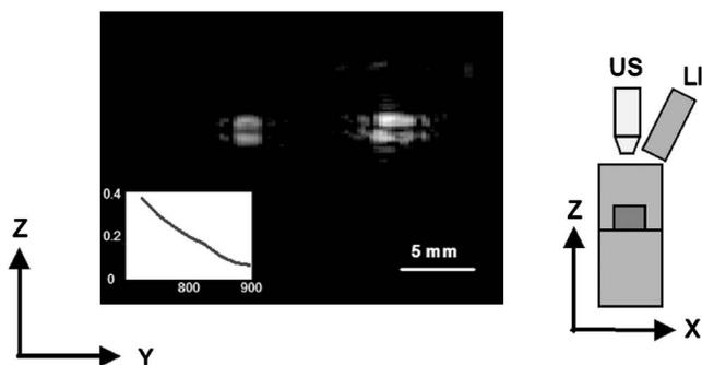
FIG. 3. (Left) Photoacoustic image of a phantom object at illumination wavelength of 725 nm with two different concentrations of gold nanorods:  $6.5 \times 10^{11}$  (right) and  $2.6 \times 10^{10}$  (left) nanoparticles/ml. (Right) Imaging setup including the fiber bundle line illuminator (IL), the ultrasound probe (US), and the phantom object.
