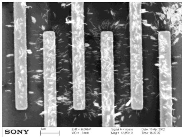
**Figure 2.** Electrically aligned ZnO nanorods between 800-nm spaced, interdigitated gold electrodes on silicon oxide. The electrode fingers on the bottom and on the top were on the same potential. The applied electric field strength was  $1.25 \times 10^7$  V/m, and the frequency was 1 kHz.
