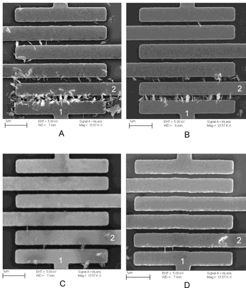
**Figure 3.** Electrically aligned ZnO nanorods between 200-nm spaced gold electrodes. The applied electric field strength was  $1.25 \times 10^7$  V/m, and the frequency was 10 kHz. The following concentrations were used: (A) ZnO nanorod stock concentration of approximately 1 mM (sample 1); (B) 50% diluted stock in ethylene glycol/water (sample 2); (C) and (D) 66% diluted stock (samples 3 and 5).
