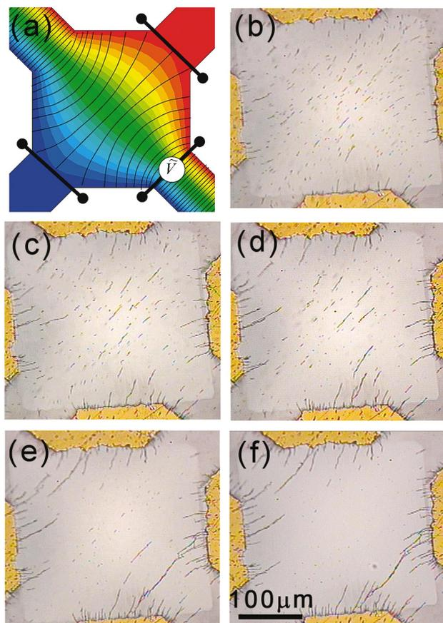
FIG. 2. (Color) (a) Simulated potential (in color contour) and electric field (in black lines) in a quadrupole with connected pairs of electrodes. Images of nanowires at (b) 2, (c) 6, (d) 10, (e) 59, and (f) 180 s after 10 V at 1 MHz has been applied.
