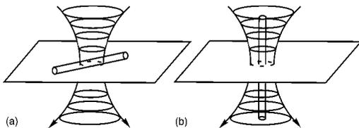
FIG. 2. A sketch of the orientations possible for nanorods described here. The nanorods are trapped in a focused Gaussian beam propagating down. In (a), the nanorod is transversely oriented with respect to the light propagation axis. In (b), the nanorod is axially oriented.
