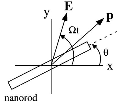
FIG. 3. A sketch of the light torque geometry. Here the induced dipole  $\mathbf{p}$  will move to align with the electric field  $\mathbf{E}$  to minimize energy. Hence, a torque  $\boldsymbol{\tau} = \mathbf{p} \times \mathbf{E}$  exists about an axis out of the plane of the paper. The light propagation direction is into the paper.
