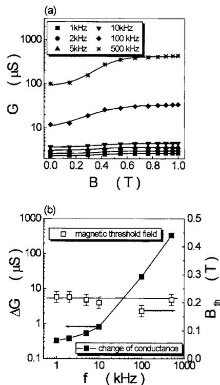
FIG. 3. (a) Device performance as a function of applied probe frequency  $f$ . (Note the logarithmic scales). (b) The change in conductance  $\Delta G$  increases with applied frequency (closed squares), while the magnetic threshold field  $B_{\text{th}}$  is practically constant (open squares).
