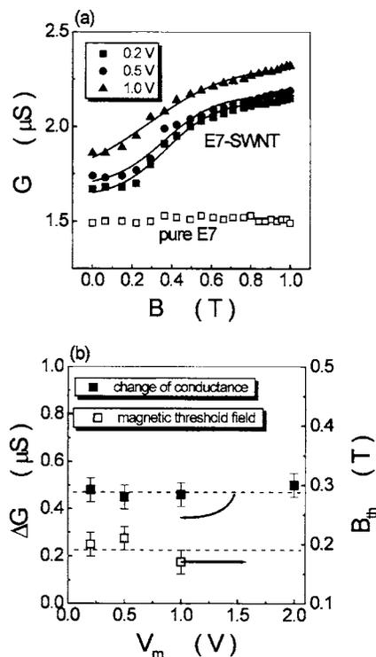
FIG. 2. (a) Device performance as a function of applied electric probe voltage  $V_m$ . (b) The change of conductance  $\Delta G$  (closed squares) and the magnetic threshold field  $B_{\text{th}}$  (open squares) is independent of the probe voltage.
