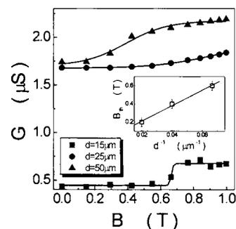
FIG. 4. Device performance for cells of different gaps between  $15\text{--}50\ \mu\text{m}$ . The inset demonstrates the linear dependence of the magnetic threshold  $B_{\text{th}}$  on reciprocal cell gap  $d^{-1}$ .
