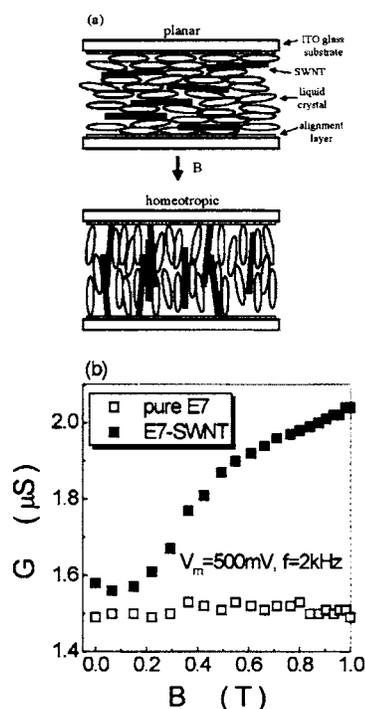
FIG. 1. (a) Schematic illustration of the working principle of the magnetically steered LC-single-wall nanotube dispersion device. (b) Experimental verification of the device, showing the conductance  $G$  of the pure LC (open squares) and the nanotube dispersed material (closed squares) as a function of applied magnetic field  $B$  for a probe voltage of  $V_m=0.5$  V at frequency  $f=2$  kHz.
