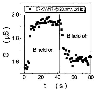
FIG. 5. Dynamic response of the magnetically steered LC-nanotube device. The characteristic decay time is found to be  $\tau=(4.0\pm 0.6)$  s.
