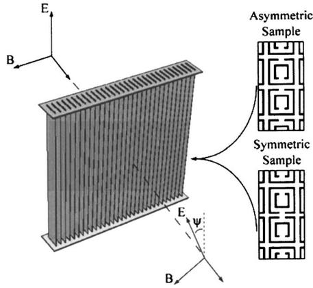
FIG. 5. Schematic diagram of the 0° SRR medium sample.
