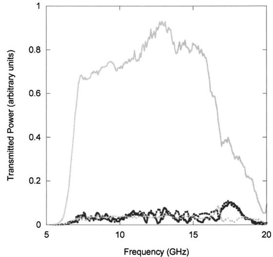
FIG. 9. Comparison of cross-polarization measurements for the symmetric  $0^\circ$  SRR medium (black dashed curve) and the symmetric  $45^\circ$  SRR medium (solid black curve). The transmission (solid gray curve) is shown again for no sample present, horns aligned. The dashed gray line corresponds to the asymmetric  $45^\circ$  SRR medium with alternating planes.
