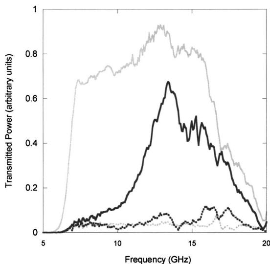
FIG. 8. Comparison of cross-polarization measurements for the asymmetric  $0^\circ$  SRR medium (black dashed curve) and the asymmetric  $45^\circ$  SRR medium (solid black curve). For calibration, measurements of the transmission with horns aligned (solid gray curve) and cross polarization (dashed gray curve) are shown for no sample present. The shape of the solid gray curve is set by the characteristics of the standard gain X-band microwave horn used in the experiments.
