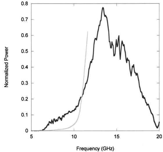
FIG. 10. Comparison of predicted cross polarization with the measured data, asymmetric  $45^\circ$  sample. Both the measured data and calculated curve are normalized such that a value of 1 indicates 100% cross polarization.
