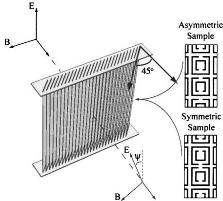
FIG. 7. Schematic of the  $45^\circ$  SRR medium sample.
