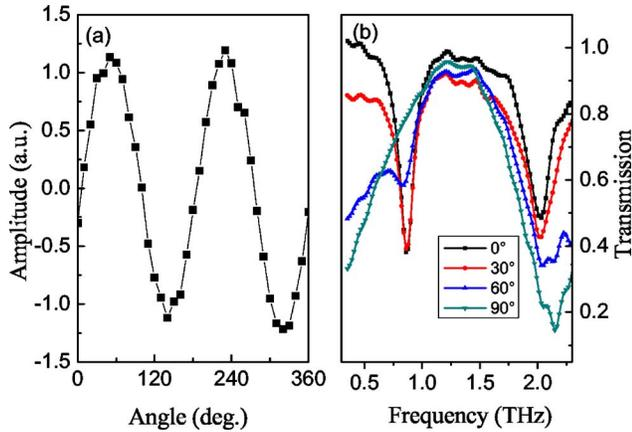
Fig. 3. (Color online) (a) Angular dependence of the transmission of a THz peak signal through the in-plane SRR-wire metamaterials. (b) Transmission through the in-plane SRR-wire metamaterials as a function of frequency at different polarization orientations ( $0^\circ$ ,  $30^\circ$ ,  $60^\circ$ , and  $90^\circ$ ).
