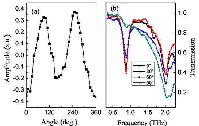
Fig. 2. (Color online) (a) Angular dependence of the transmission of a THz peak signal through the SRR sample. (b) Transmission through the SRR sample as a function of frequency at different polarization orientations ( $0^\circ$ ,  $30^\circ$ ,  $60^\circ$ , and  $90^\circ$ ).
