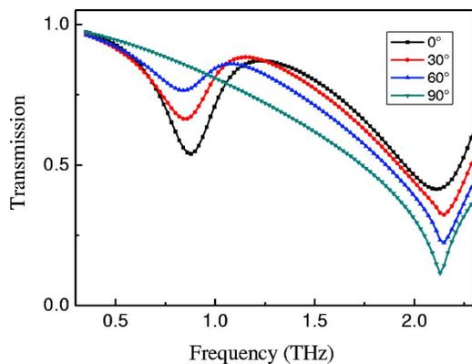
Fig. 4. (Color online) Simulation of the transmission through the SRR sample as a function of frequency at different polarization orientations ( $0^\circ$ ,  $30^\circ$ ,  $60^\circ$ , and  $90^\circ$ ).
