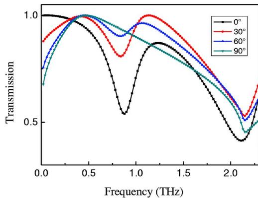
Fig. 5. (Color online) Simulation of the transmission through the in-plane SRR-wire metamaterials as a function of frequency at different polarization orientations ( $0^\circ$ ,  $30^\circ$ ,  $60^\circ$ , and  $90^\circ$ ).
