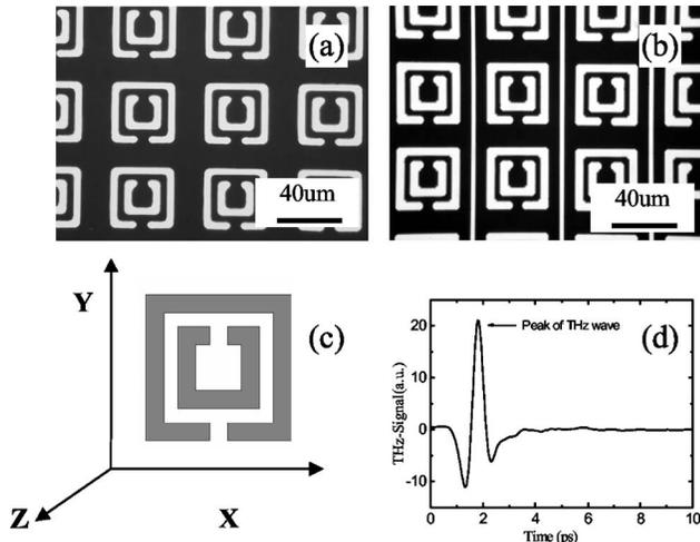
Fig. 1. (a) Schematic of a SRR on a quartz slab. (b) Schematic of in-plane SRR-wire metamaterials on a quartz slab. (c) The Cartesian coordinate system  $(x,y,z)$  is chosen in our experiment with the sample located in the  $x,y$  plane and the incident wave is along the  $z$  axis. The electric vector is along the  $x$  axis. The gap-bearing sides of the SRR is along the  $x$  axis. (d) Typical THz time-domain wave; the arrow indicates the peak of the THz wave.
