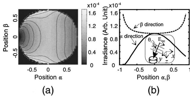
Fig. 5. Distribution of light diffracted by a small dielectric disk: (a) irradiance distribution, (b) cross section of (a). The diameter and the thickness of the disk are  $\lambda/2$  and  $\lambda/50$ , respectively. The refractive index of the disk is 2.15. The incident light is linearly polarized, and the incident angle is  $64^\circ$  ( $p$  polarization).
