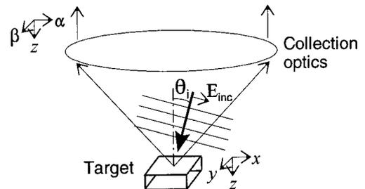
Fig. 1. Layout of the target and the collection optics assumed in the calculations.
