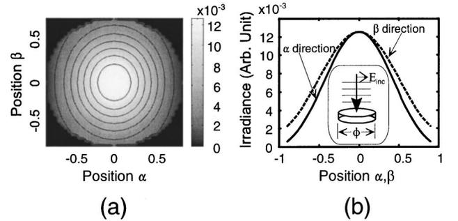
Fig. 3. Distribution of light diffracted by a large dielectric disk: (a) irradiance distribution, (b) cross section of (a). The diameter and the thickness of the disk are  $\lambda$  and  $\lambda/50$ , respectively. The refractive index of the disk is 2.15. The incident light is linearly polarized, and the incident angle is  $0^\circ$ .
