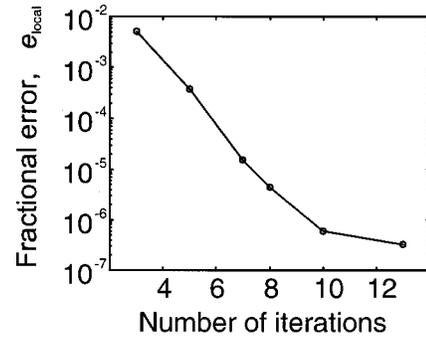
Fig. 11. Dependence of the error  $e_{\text{local}} \equiv |A \times P - E_{\text{incl}}|/|E_{\text{incl}}|$  on the number of iterations for a small dielectric disk. The diameter and the thickness of the disk are  $\lambda/2$  and  $\lambda/50$ , respectively. The refractive index of the disk is 2.15. The incident light is linearly polarized, and the incident angle is  $0^\circ$ .
