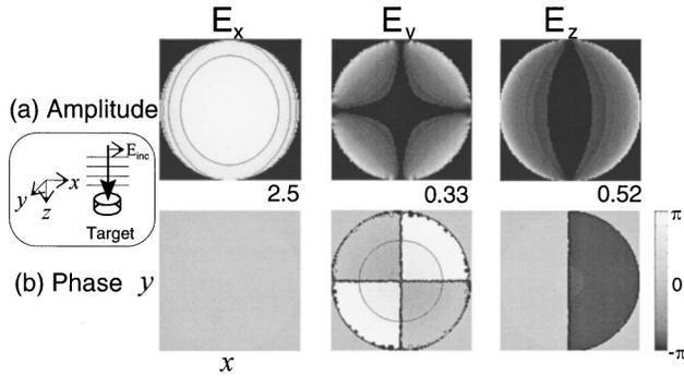
Fig. 9. Electric field distribution at a top surface of a small dielectric disk: (a) amplitude for  $x$ ,  $y$ , and  $z$  components; (b) phase corresponding to (a). The diameter and the thickness of the disk are  $\lambda/2$  and  $\lambda/50$ , respectively. The refractive index of the disk is 2.15. The incident light is linearly polarized, and the incident angle is  $0^\circ$ .
