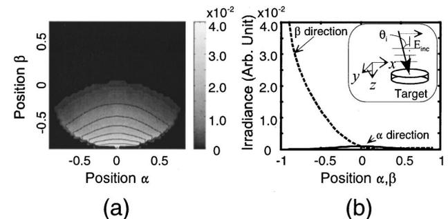
Fig. 8. Distribution of light diffracted by a large dielectric disk: (a) irradiance distribution, (b) cross section of (a). The diameter and the thickness of the disk are  $\lambda$  and  $\lambda/50$ , respectively. The refractive index of the disk is 2.15. The incident light is linearly polarized, and the incident angle is  $64^\circ$  ( $s$  polarization).
