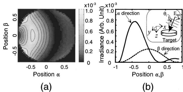
Fig. 6. Distribution of light diffracted by a large dielectric disk: (a) irradiance distribution, (b) cross section of (a). The diameter and the thickness of the disk are  $\lambda$  and  $\lambda/50$ , respectively. The refractive index of the disk is 2.15. The incident light is linearly polarized, and the incident angle is  $64^\circ$  ( $p$  polarization).
