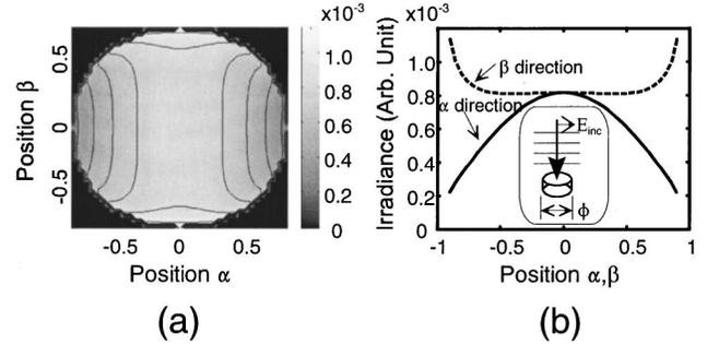
Fig. 2. Distribution of light diffracted by a small dielectric disk: (a) irradiance distribution, (b) cross section of (a). The diameter and the thickness of the disk are  $\lambda/2$  and  $\lambda/50$ , respectively. The refractive index of the disk is 2.15. The incident light is linearly polarized, and the incident angle is  $0^\circ$ .
