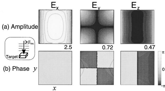
Fig. 10. Electric field distribution at a top surface of a small dielectric square plate: (a) amplitude for  $x$ ,  $y$ , and  $z$  components, (b) phase corresponding to (a). The size of a side and the thickness of the square are  $\lambda/2 \times \lambda/2$  and  $\lambda/50$ , respectively. The refractive index of the plate is 2.15. The incident light is linearly polarized, and the incident angle is  $0^\circ$ .
