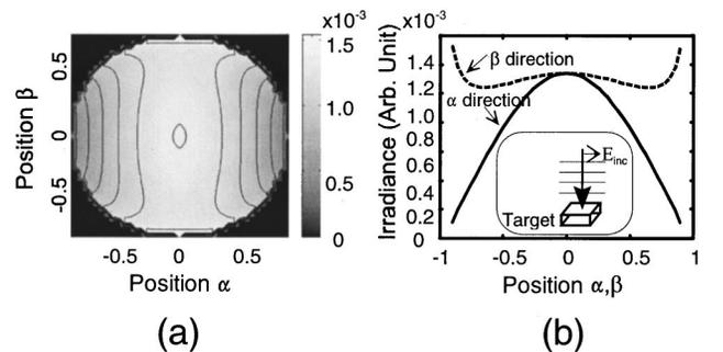
Fig. 4. Distribution of light diffracted by a small dielectric square plate: (a) irradiance distribution, (b) cross section of (a). The length of a side and the thickness of the square are  $\lambda/2 \times \lambda/2$  and  $\lambda/50$ , respectively. The refractive index of the plate is 2.15. The incident light is linearly polarized, and the incident angle is  $0^\circ$ .
