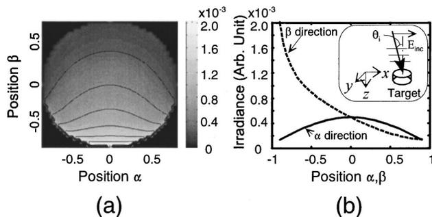
Fig. 7. Distribution of light diffracted by a small dielectric disk: (a) irradiance distribution, (b) cross section of (a). The diameter and the thickness of the disk are  $\lambda/2$  and  $\lambda/50$ , respectively. The refractive index of the disk is 2.15. The incident light is linearly polarized, and the incident angle is  $64^\circ$  ( $s$  polarization).
