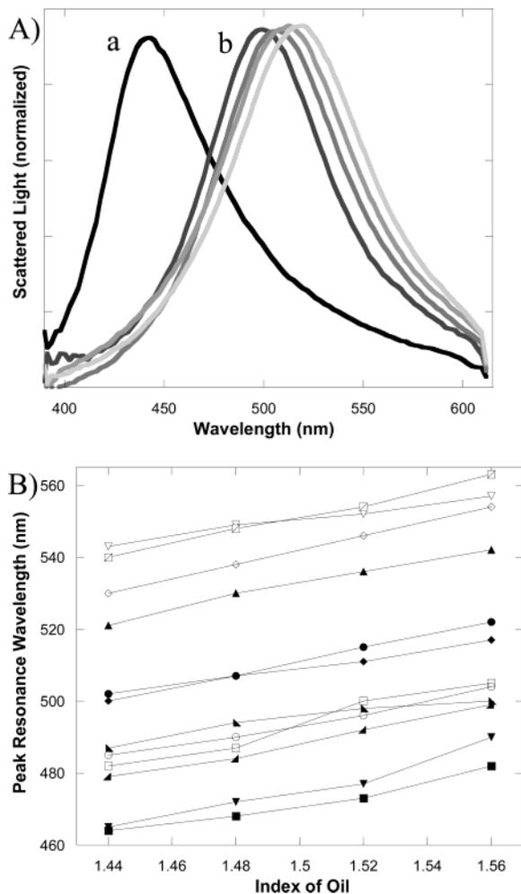
**Figure 2.** Spectral shift for individual blue (roughly spherical) silver nanoparticles. (A) Typical blue particle spectrum as it is shifted from (a) air to (b) 1.44 index oil, and successive oil treatments in 0.04 index incremental increases. (B) Peak spectral position vs index of oil applied to 12 individual blue (roughly spherical) particles studied. The average slope of the linear fit to these curves suggests a 1.6 nm red shift per 0.01 index increase.
