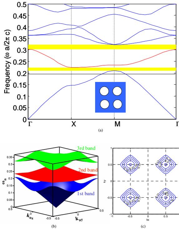
Fig. 2. (a) TE mode dispersion diagram of the square-lattice PhC. (b) TE mode photonic band structure of the square-lattice PhC. (c) TE mode EFCs of the square-lattice PhC at the vicinity of the first bandgap.
