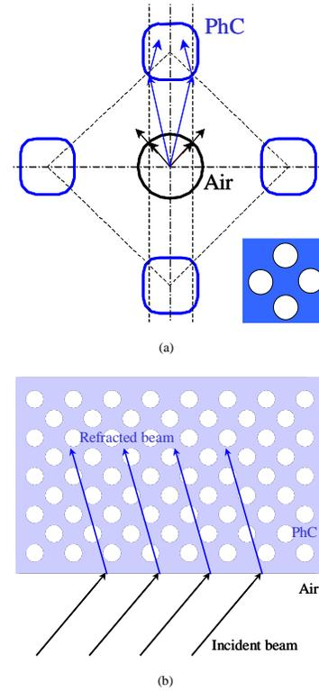
Fig. 3. (a) Illustration of propagation of the incident beam and refracted beam in  $k$ -space. (b) Illustration of propagation of the incident beam and refracted beam in real space.
