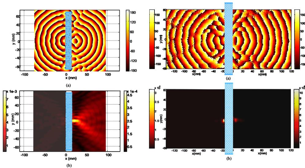
Fig. 4. (a) Simulated phase distribution (unit: radian) when a dipole is placed at object distance  $1\text{mm}$ : TE mode at  $24.6\text{GHz}$ . (b) Simulated amplitude distribution when a dipole is placed at object distance  $1\text{mm}$ : TE mode at  $24.6\text{GHz}$ .
