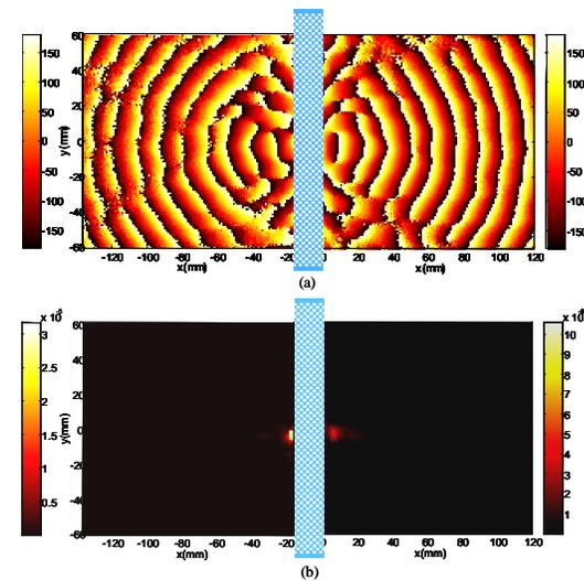
Fig. 5. (a) The measured phase distributions (in degrees) at  $23.2\text{GHz}$  for the source (left) and the image (right). The flat lens (photonic crystal) is depicted between the source and the image. (b) The measured amplitude distributions at  $23.2\text{GHz}$ . The flat lens (photonic crystal) is depicted between the source and the image.
