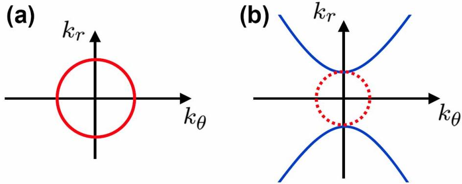
Fig. 3. Dispersion relation for isotropic medium (a) and for a material with  $\epsilon_r < 0$ ,  $\epsilon_\theta > 0$  (b). Note that for a fixed frequency, the wave vector  $k$  can take on arbitrarily large values (within the effective medium approximation).
