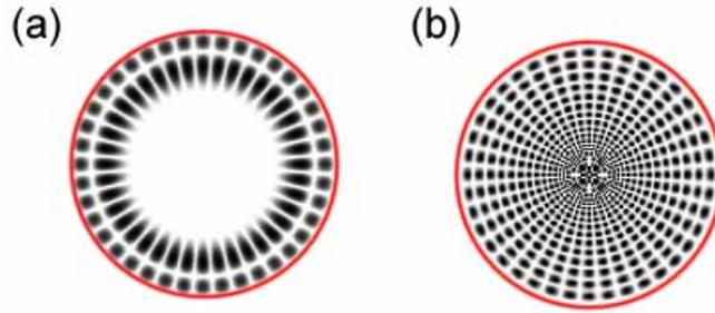
Fig. 4. (a) High angular momentum states in an isotropic dielectric cylinder (b) High angular momentum states in a cylinder made of  $\epsilon_\theta > 0$ ,  $\epsilon_r < 0$  metamaterial (in the effective medium approximation); note that the field penetrates to the center.
