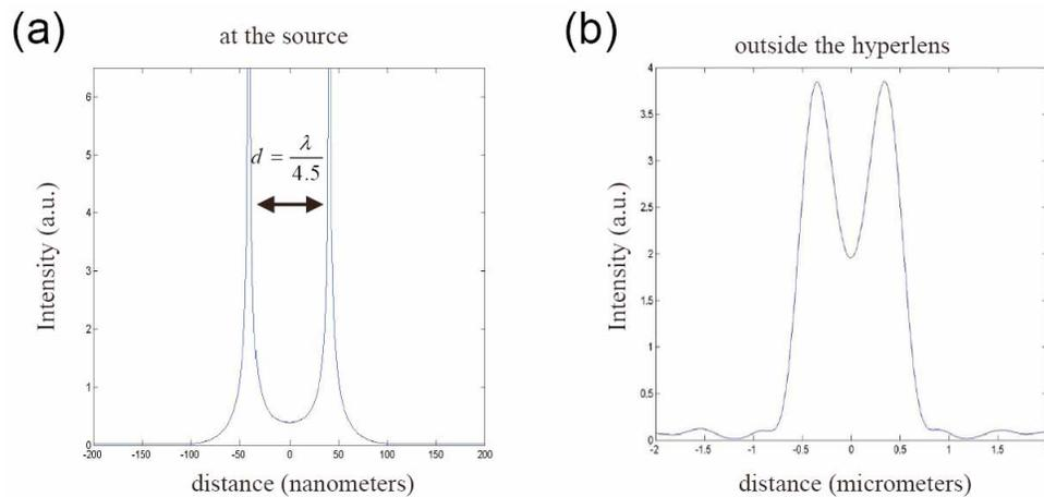
Fig. 8. Demonstration of subwavelength resolution in the composite hyperlens containing two sources placed a distance  $\lambda/4.5$  apart inside the core. (a): Field at the source. (b): Field outside the hyperlens.
