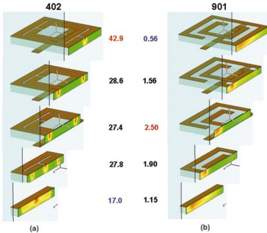
FIG. 2. (Color) Simulated (using EBC, MBC) power loss density for (a) the 402 structure and (b) the 901 structure. The 901 structure does not have the additional wire at the bottom of the 901 HWD unit cell as shown in Fig. 1. The numbers in the diagram indicate the maximum power loss density (a.u.) at each cut plane. For the 402 structure,  $C=0.025$  cm,  $D=0.0075$  cm,  $G=0.010$  cm,  $H=0.0254$  cm,  $L=0.33$  cm,  $S=0.215$  cm, and  $T=17 \times 10^{-4}$  cm.
