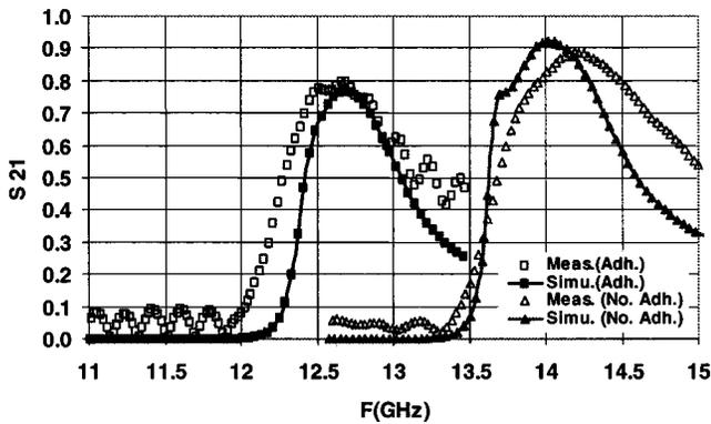
FIG. 4. Measured (open points) and simulated (solid points)  $S_{21}$  scattering parameters for 901 HWD structure with and without a 0.010 cm adhesive holding adjacent layers of NIM unit cells together. The simulations used PBC corresponding to the actual experimental samples. The adhesive had an  $\epsilon = 2.68$  and  $\tan \delta = 0.016$ .
