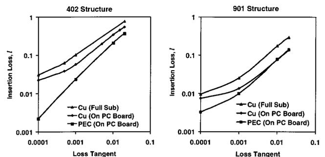
FIG. 3. Simulated (using EBC, MBC) losses at the passband peak for the (a) 402 and (b) 901 structures. Cu (full sub) stands for Cu embedded in a solid dielectric unit cell, whereas the Cu (on PC board) refers to a copper pattern on top of a substrate surrounded by air. PEC stands for a perfect electrical conductor.
