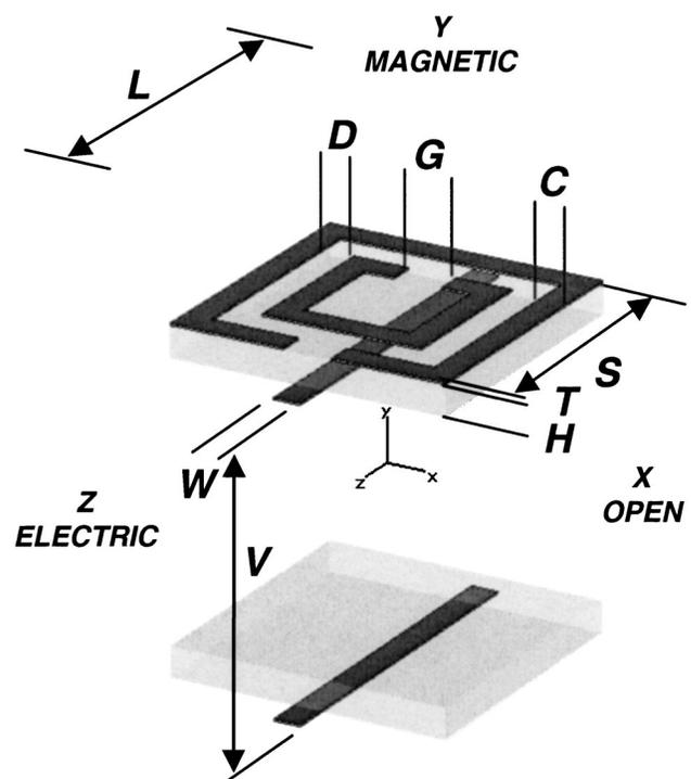
FIG. 1. Unit cell showing EBC, MBC, and the dimensions of the 901 HWD structure examined in this study. The direction of propagation of the electromagnetic field is along the  $x$  axis, the electric field along the  $z$  axis, and the magnetic field along the  $y$  axis. For the 901 HWD structure  $C = 0.025$  cm,  $D = 0.030$  cm,  $G = 0.046$  cm,  $H = 0.0254$  cm,  $L = 0.33$  cm,  $S = 0.263$  cm,  $T = 17.0 \times 10^{-4}$  cm,  $W = 0.025$  cm, and  $V = 0.255$  cm.
