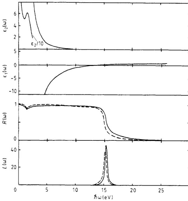
**Figure 2.** Optical properties of aluminium: full curves, calculations; broken curves, measurements of  $R(\omega)$  and  $L(\omega) = \text{Im}(-1/\epsilon(\omega))$  (from Shiles *et al* 1980) (arbitrary units).
