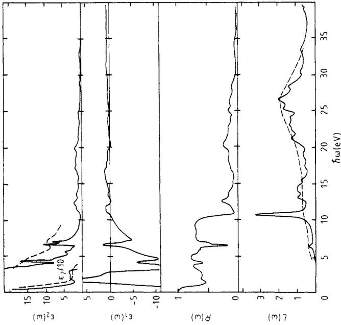
**Figure 12.** Optical properties of chromium: full curves, calculations; broken curves, measurements of  $\epsilon_1(\omega)$  (from Nestell and Christy 1980) and  $L(\omega)$  (from Misell and Atkins 1973) (arbitrary units).
