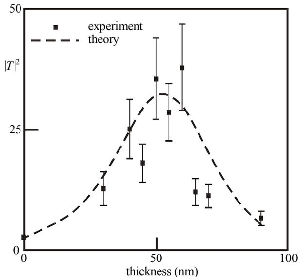
**Figure 5. Amplifying the near field:** near fields incident on thin films of silver are transmitted to the far side with amplification, at least up to a critical thickness. For thicker films losses dominate and spoil the resonant effect. Data taken from a paper by Fang *et al.*<sup>11</sup>.
