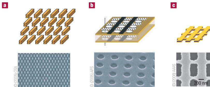
**Figure 3** Different designs of metamaterials at optical frequencies. a–c, as reported in refs 4 (a), 5 (b) and 6 (c). The top row shows the schematic representations of the different ‘meta-atoms’, with microscope images of the actual samples below.
