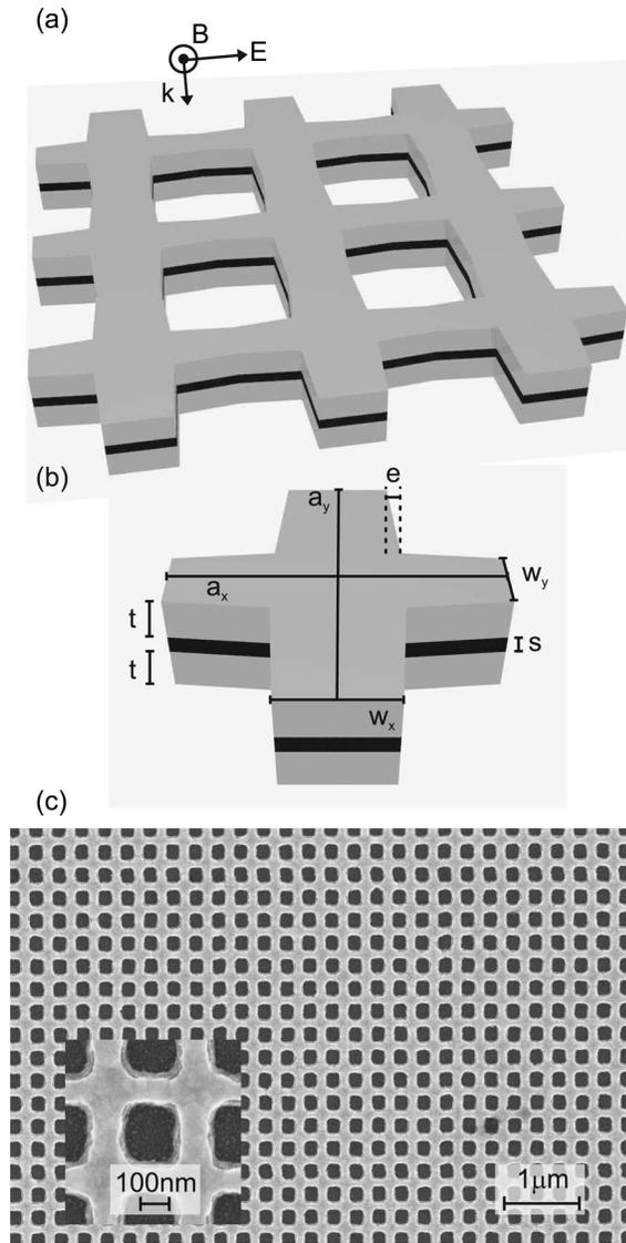
Fig. 1. (a) Scheme of the metamaterial and polarization configuration. (b) Unit cell of the structure with definition of parameters: lattice constant  $a_x = a_y = 300$  nm,  $w_x = 102$  nm,  $w_y = 68$  nm,  $t = 40$  nm,  $s = 17$  nm, and  $e_x = e_y = e = 8$  nm. The last parameter describes small deviations from rectangular shape. (c) Top-view electron micrograph of the sample employed in Figs. 2 and 3. Inset, magnified view.
