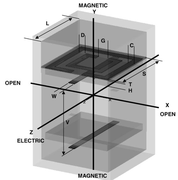
FIG. 1. Unit cell of the 901 HWD structure used in the numerical simulations. The direction of propagation of the electromagnetic field is along the  $x$  axis, the electric field is oriented along the  $z$  axis, and the magnetic field is along the  $y$  axis.  $C = 0.025$  cm,  $D = 0.030$  cm,  $G = 0.046$  cm,  $H = 0.0254$  cm,  $L = 0.33$  cm,  $S = 0.263$  cm,  $T = 17.0 \times 10^{-4}$  cm,  $W = 0.025$  cm, and  $V = 0.255$  cm.
