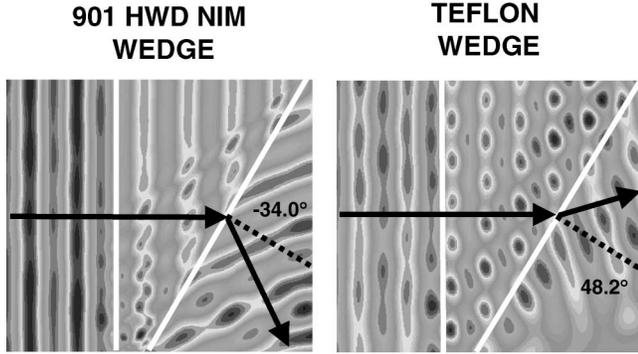
FIG. 3. Contour plots, in the  $z = 0$  plane (medium plane of the experiment), of the  $E_z$  component of the electric field as computed by MAFIA at 12.6 GHz. The radiation propagates from left to right. The wedge angle is  $32.19^\circ$ . Left: NIM wedge  $n = \{-1.0454 - 0.0041i\}$  ( $i, \epsilon = \{1, 1, -1.8922 - 0.0001i\}$ ,  $\mu = \{1, -0.5775 - 0.0045i, 1\}$ ). Right: Teflon wedge  $n = 1.4$ .
