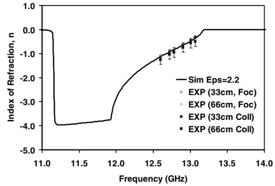
FIG. 7. Experimental and computed dispersion relation of the index of refraction for the 901 HWD structure with substrate  $\epsilon = 2.2$ . The experimental data were taken in both the focused and collimated beam setup at 33 and 66 cm from the wedge.
