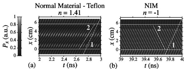
FIG. 4. Plots  $P_x(x, y = 0, z = 0, t)$  showing contours of constant phase velocity simulations for (a) the Teflon wedge and (b) the NIM wedge. The solid horizontal lines denote the edges of the wedge, and the dashed lines highlight the fringe slopes that represent the phase velocities: (1) corresponds to  $c$ , the phase velocity in vacuum; (2) corresponds to  $c/n$ , the phase velocity in the respective materials.
