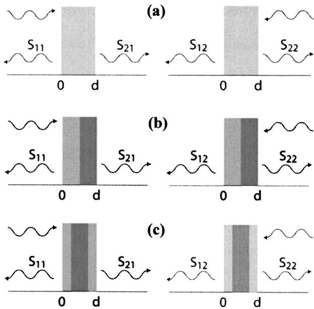
FIG. 1.  $S$ -parameter measurements on (a) a homogeneous 1D slab; (b) an inhomogeneous asymmetric 1D slab; and (c) a symmetric inhomogeneous 1D slab. The parameter  $d$  represents the thickness of a single unit cell of the structure. The different shaded regions represent different homogeneous materials, each with distinct values of material parameters.
