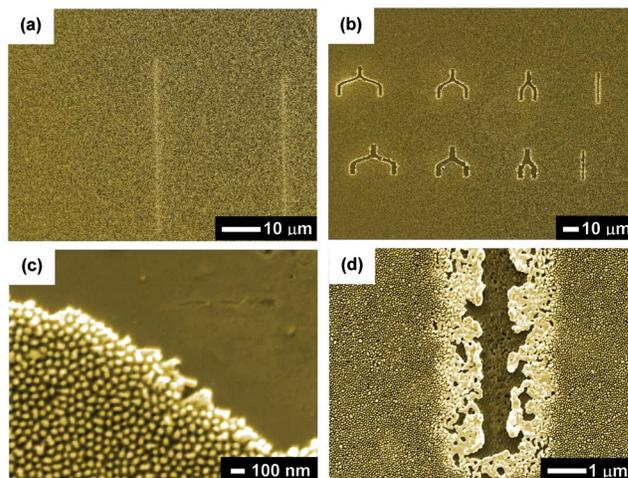
FIG. 4. (Color online) SEM images of the structures created by (a) melting and (b)–(d) ablation of the nanorods. The pulse energy is 0.25 nJ in (a) and 80 nJ in (b) and (c) and 120 nJ in (d).
