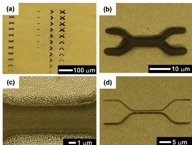
FIG. 2. (Color online) Scanning electron microscopy (SEM) images of the polymer structures created onto the nanorod arrays. (a) Various structures written with different laser light intensities. The intensity decreases from 16 to 10 mW when moving from top to bottom. (b)–(d) zoom into the images. The structure in (b) and (c) has been written with 16 mW and in (d) with 10 mW laser power.
