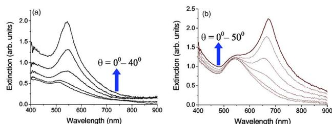
FIG. 3. (Color online) Extinction spectra of the Au nanorods (length of 350 nm, diameter of 25 nm, and spacing of 40 nm) in the region without (a) and with (b) polymer present measured at different angles of incidence (changed in  $10^\circ$  steps) of *p*-polarized light.
