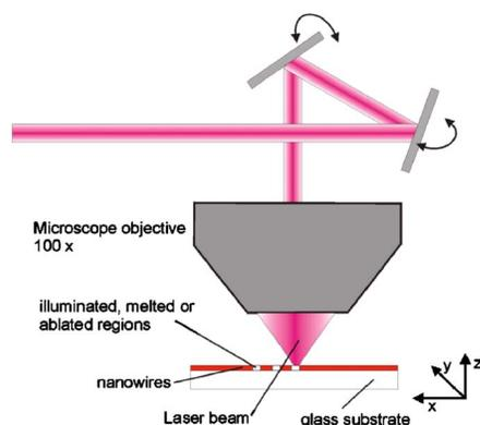
FIG. 1. (Color online) Schematics of the femtosecond laser writing setup used for the restructuring of nanorod arrays. Computer-controlled rotating mirrors are used for the steering of the laser beam during writing.
